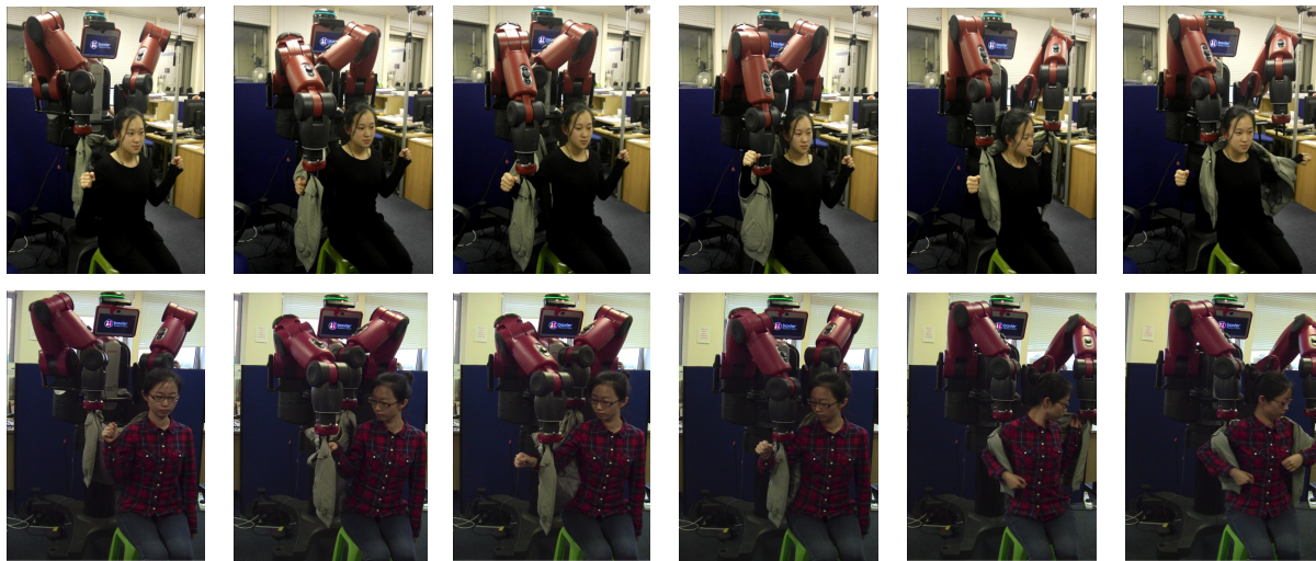
Fig. 5: Sequential shots of personalised assistive dressing. A Baxter robot assists two users to wear a sleeveless jacket individually. The robot motions are planned according to the user models and real-time upper-body pose.
